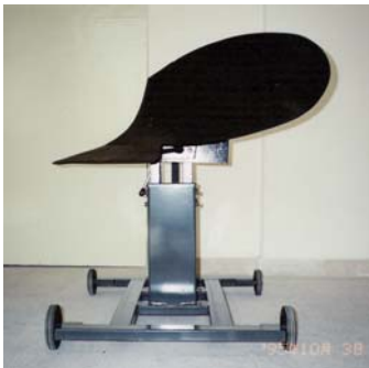
Fig. 12 - Adjusting the mouldboard on the support for horizontal and vertical positions
