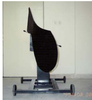
Fig. 12 - Adjusting the mouldboard on the support for horizontal and vertical positions
