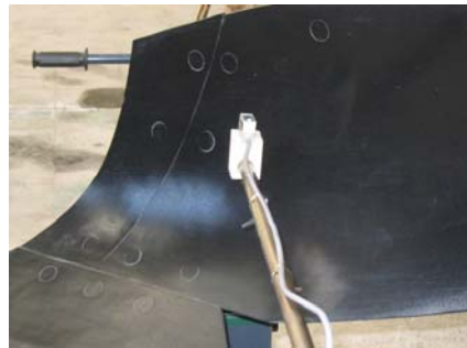
Fig. 8 - Working mechanism of movable ruler and drawer rod with optical sensor
