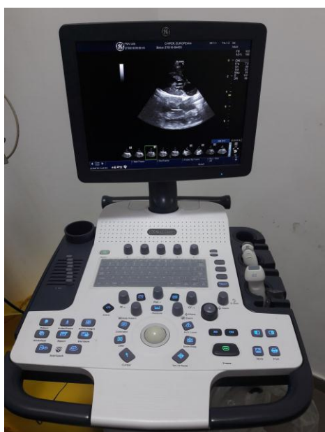
Fig.5.2. Ecograful General Electric Logiq V5 Expert dotat cu sonda phased array 4-10 MHz.
