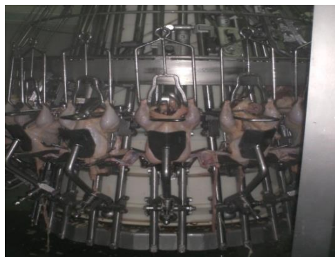
Figura 2. 13 Sistem automat de eviscerare Figure 2.13 Automatic bird evisceration system
