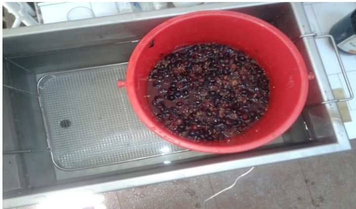
Figura nr. 3.5. Baie de ultrasunete Bandelin Sonorex®, modelul RK 1028 (original) Figure no. 3.5. Bandelin Sonorex® ultrasonic bath, model RK 1028 (original)
