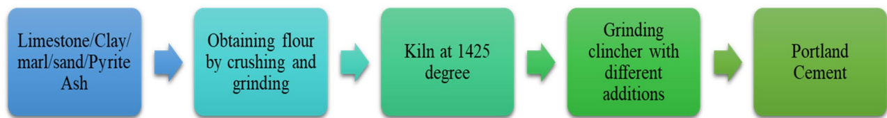
Fig. 14. Production stages for ordinary Portland cement.
