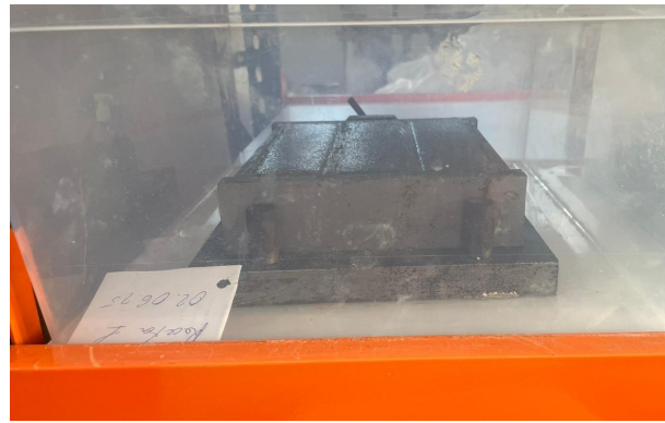
Figure 8. Drying of mortar samples drying process.
