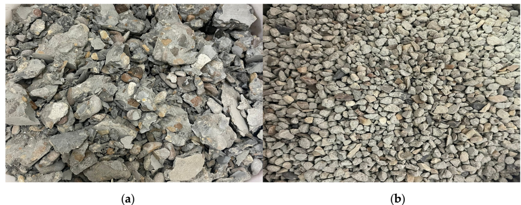
Figure 5. Demolition concrete waste aggregates: (a) crushed concrete (b) big sieve.
