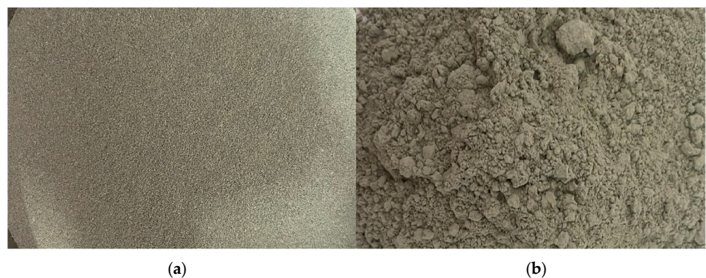
Figure 6. Recycled waste concrete aggregate: (a) small sort (b) fine part.
