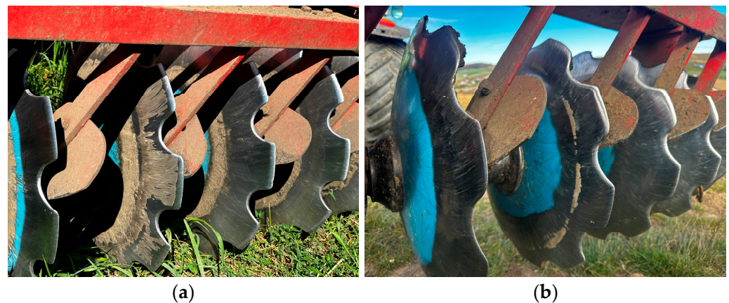
Figure 12. Field wear appearance of control sample, sample 1, sample 2, sample 3 from left to right. (a) After 25 ha per disc; (b) After 50 ha per disc.
