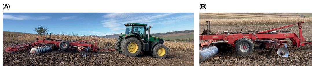
Figure 6. Disc harrow and tractor during field operation in stubble conditions. (A) Overview of the tractor and the 4 m disc harrow; (B) close-up side view with the implement in operation.
