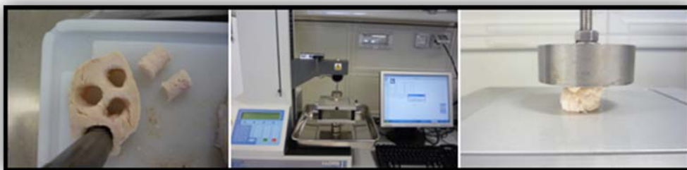
Fig. 4.12 Determinarea texturii cărnii (TPA) Fig. 4.12 Determination of meat texture (TPA)
