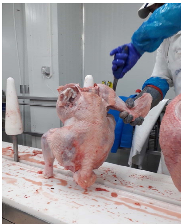
Figura 6.14 Tranșarea aripilor Figure 6.14 Portioning of wings
