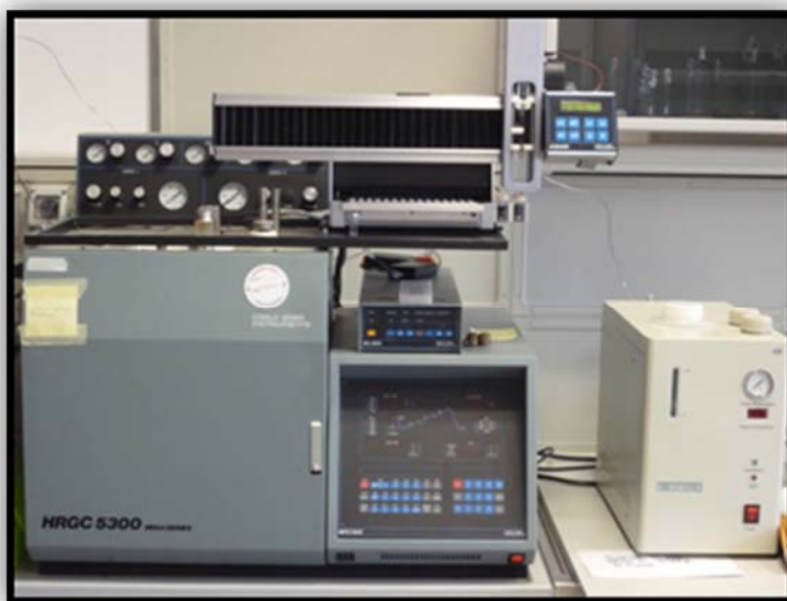
Fig. 4.15 Gaz-cromatograful GC Carlo Erba 5300 mega series Fig. 4.15 GC Carlo Erba 5300 mega series gas-chromatography
