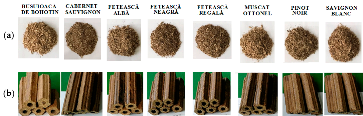
Figure 4. Pictures with: (a) dried and ground biomass before densification; and (b) obtained briquettes.
