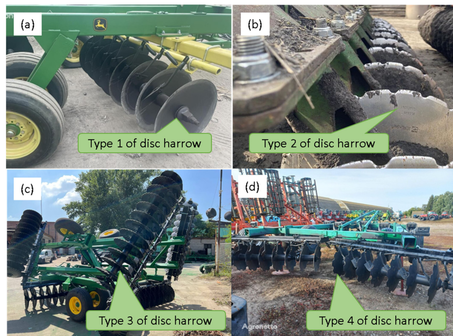
Figure 1. Different types (geometrical forms) of discs in the disc harrow assembly. (a). Single-action disc harrow. (b) Notched edge with small profile. (c). Double-action disc harrow (d). Notched edge with large profile [4,10].
