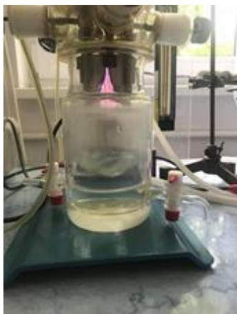
Fig. 1. Configuration of the non-thermal plasma generator based on a gliding arc discharge
