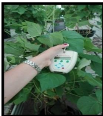
Fig. 3.13. CCM 200 plus (Chlorophyll Content Meter) (original)
