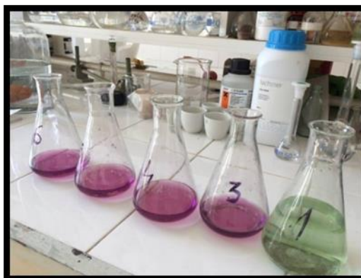
Fig. 3.22. Determinarea proteinei – titrarea (original)
