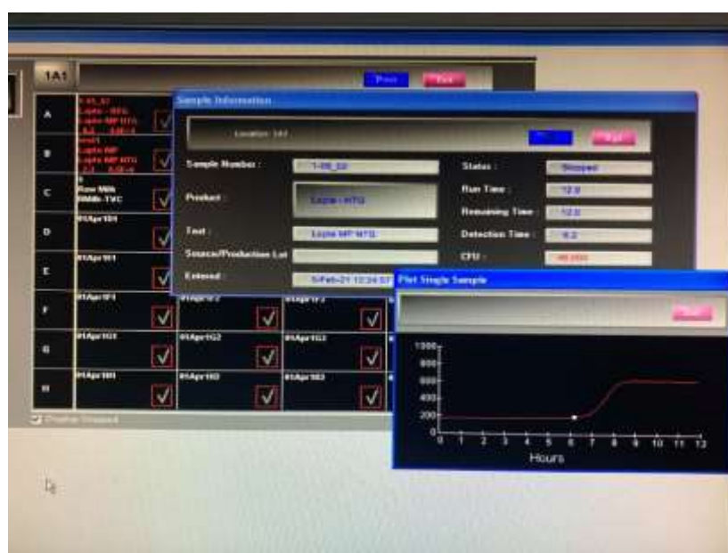
Figure 5 Graphical representation of the detection curve of the total number of germs generated in real time
