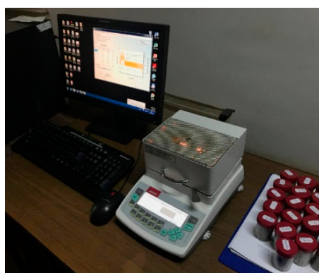
Figure 9. The equipment used for measurement of moisture content.
