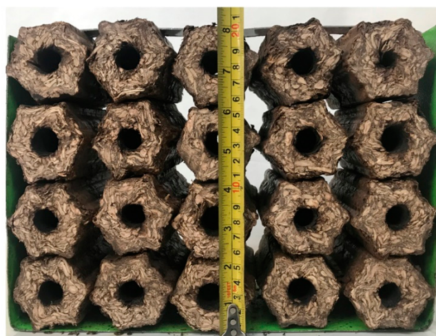
Figure 11. Evaluation of bulk density of the obtained briquettes.
