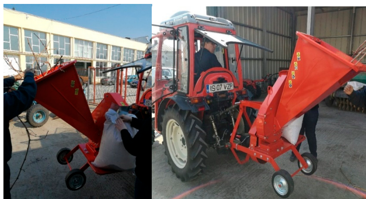
Figure 2. Operating the CARAVAGGI BIO 90 shredder used for coarse and fine grinding of the biomass.
