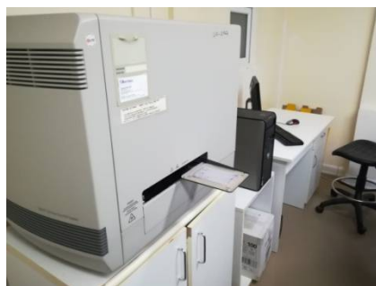
Fig. 5.3. Sistemul 7900HT Fast Real-Time PCR System (Applied Biosystems)
