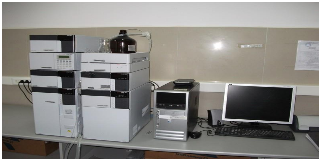
Figura 4.8 Cromatograf de lichide - SHIMADZU HPLC Prominence 2010 (original) Figure 4.8 HPLC System – Liquid Chromatography Shimadzu Prominence 2010 (original)
