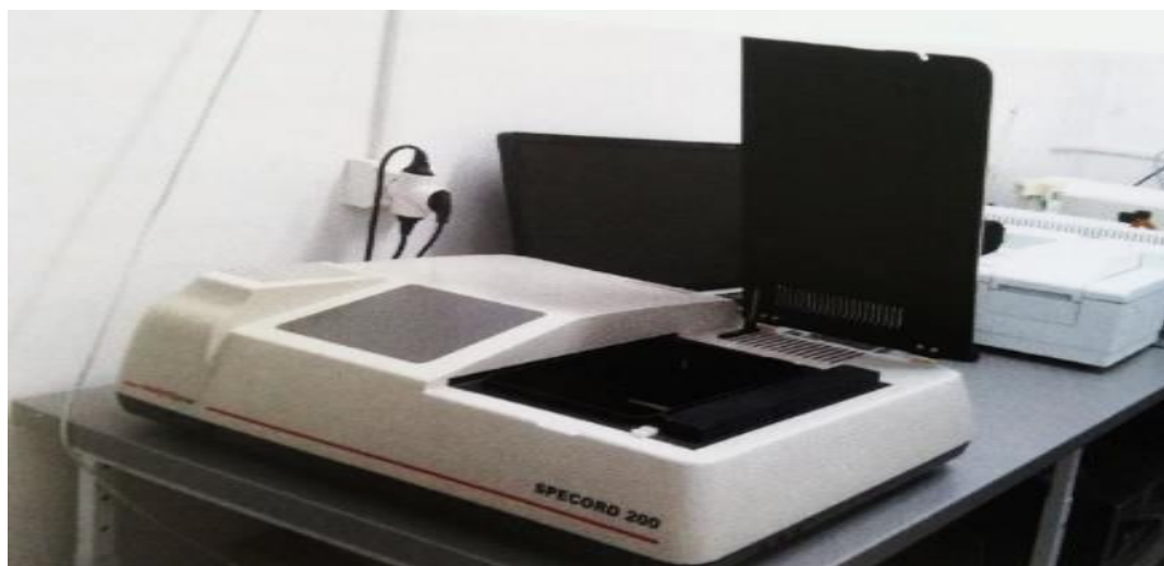
Figura 4.9 Spectofotometrul UV-VIS Analytik Jena Specord 200 (original) Figure 4.9 Spectrophotometer UV-VIS Analytik Jena Specord 200 (original)
