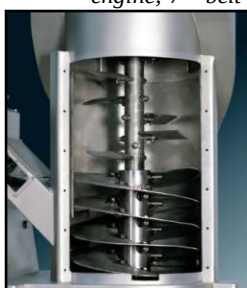
Fig. 2.15. SCV type Intensive vertical humidifier (Ocrim, 2013): A – product supply; B – product outlet; C – aspiration; 1 – arbor; 2 – profiled pallets; 3 – screw; 4 – chicanery; 5 – product detection sensor; 6 – engine; 7 – belt transmisson; 8 – rotor maintenance door; 9 – visors; 10 – frame.
