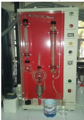
Figura 4.3 Distilator-extractor automat DUJARDIN-SALLERON DE 2000 (original) Figure 4.3 Automatic distiller-extractor DUJARDIN-SALLERON DE 2000 (original)
