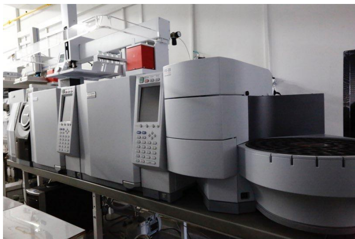
Figura 4.10 Sistem gaz-cromatografic cuplat cu spectrofotometru de masă de tip HS20-GC-MS (original) Figure 4.9 Gas-chromatographic system coupled with mass spectrophotometer HS20-GC-MS (original)
