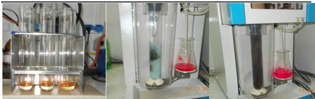
Fig. 4.6. Determinarea proteinei brute: distilarea probelor Fig.4.6. Determination of crude protein: samples distillation
