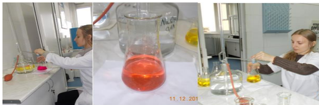
Fig. 4.7. Determinarea proteinei brute: titrarea probelor Fig.4.7. Determination of crude protein: samples titration
