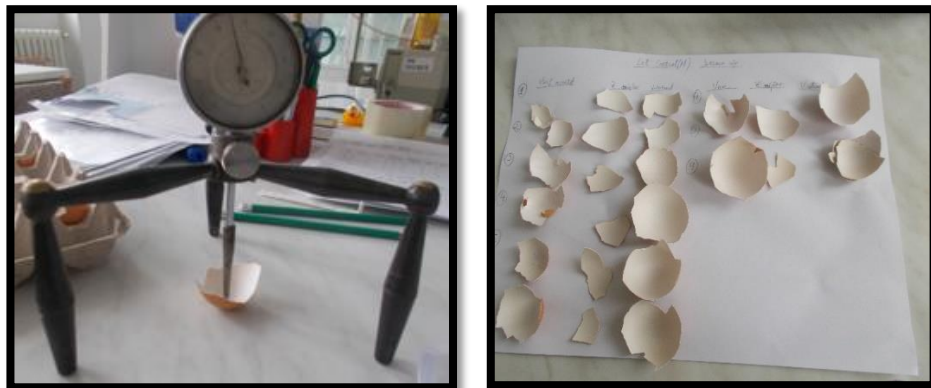
Fig. 4.22. Determinarea grosimii cojii minerale Fig.4.22. Determination of mineral shell thickness
