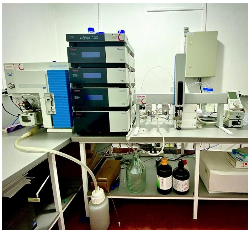
Figura 4.3 – Sistem cromatografic de tip UltiMate™ 3000 UHPLC (original) Figure 4.3 – UltiMate™ 3000 UHPLC system chromatographic (original)
