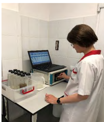
Fig.8.12. Determinare alge folosind echipamentul BBE ALA Fig. 8.12 Algae determination using the BBE ALA equipment
