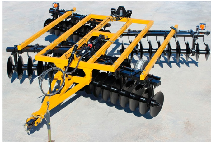
Figure 1. Double offset tandem disc harrow (four-gang configuration) used as the reference implement in this study.
