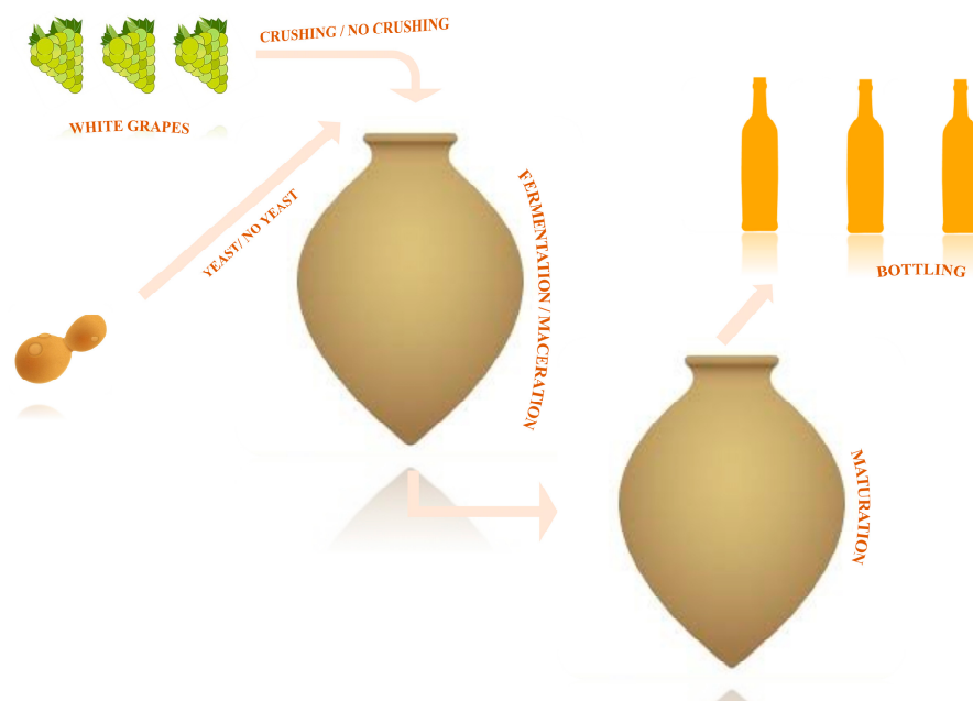
Figure 2. Basic representation of long-macerated white wine technology.
